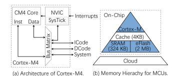
Figure 2: An illustration of the architecture and memory hierarchy for microcontrollers.
