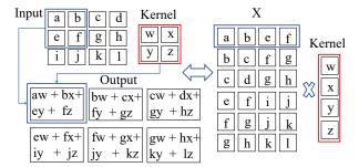
Figure 3: An illustration of convolution in deep reuse.
