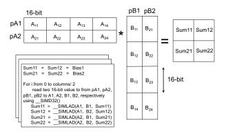
Figure 13: The demonstration of the inner loop of matrix multiplication. Each time two columns and two rows are taken into consideration.
