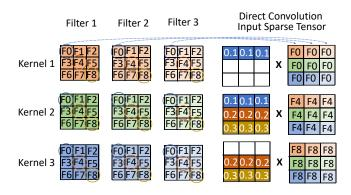
Figure 17: Direct convolution through dense matrix multiplication.
